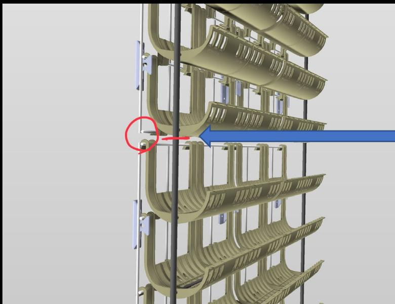
At the junction of the upper and lower kits, cut off the hose fittings and the end caps. Then connect the supply lines on both sides with the supplied  $\frac{1}{2}$ " connector fittings
