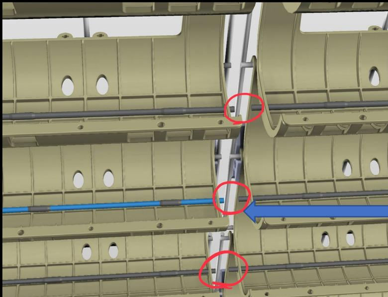
Cut off end  $\frac{1}{4}$ " end caps and connect using the  $\frac{1}{4}$ " connector fittings
